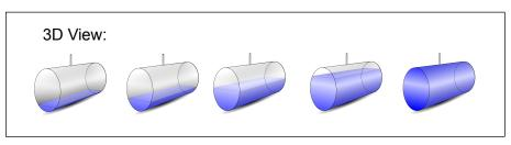
Ask students to draw the shape of surface of the water in the bottom cylinder, at five different levels.
